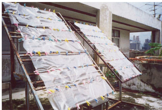
Figure 1 The exposure racks for the outdoor exposure study. [Color figure can be viewed in the online issue, which is available at www.interscience.wiley.com .]
